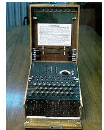
The German military used the Enigma machine during World War II for communication they thought to be secret. The large-scale decryption of Enigma traffic at Bletchley Park was an important factor that contributed to Allied victory in WWII. [13]
